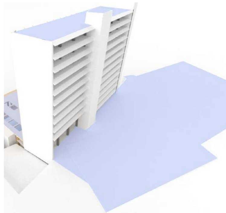
Harvesting rainwater from impermeable parking roof
